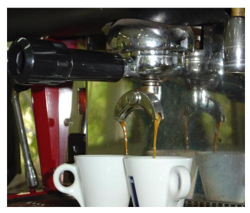
Originally an Italian specialty, Espresso is a mix of art and science. This method requires 6-7 grams of Arabica blend, grind ranging from *impalpable powder* millimeter 1 to grains, approximately 30 cc of water at  $90^{\circ}$  c and pressure 9 at
